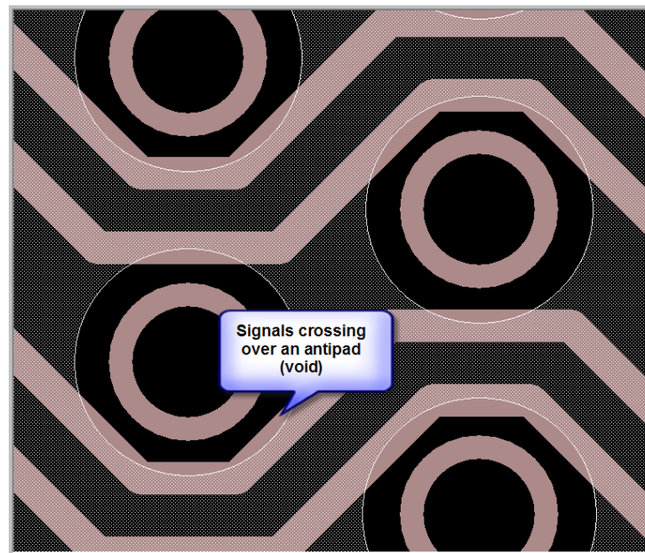
Figure 3. Signals crossing over a void in the reference plane
