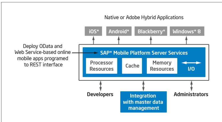
Figure 1. SAP Mobile Platform architecture
