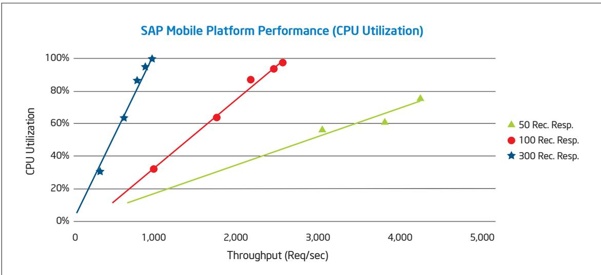
**Figure 4.** Multi-user requests results (CPU utilization)
