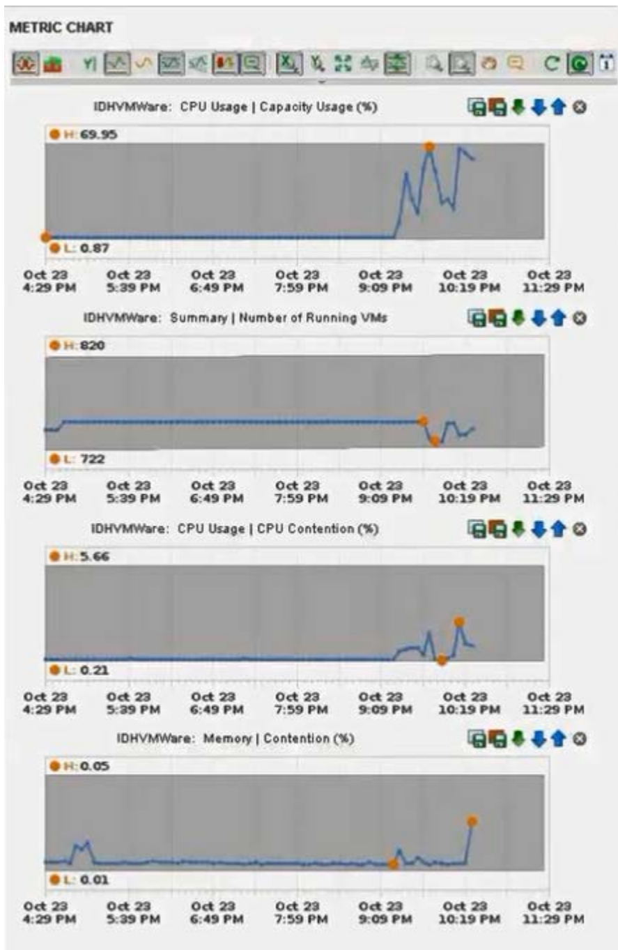
Figure 3: Performance of a heavily loaded system as seen in the vCenter Operations
