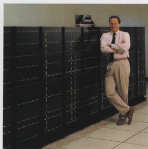
The massively parallel Touchstone Delta supercomputer uses hundreds of i860™ and i386™ CPUs to solve the most demanding computational problems. Intel Fellow Justin Rattner is the Director of Technology for the Supercomputer Systems Division.
